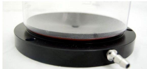
Canister and tube INCORRECTLY attached
